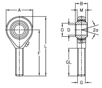
Α = 40a (degrees) = 14 В = 22 D = 17 Dynamic load C (kN) = 18.0F = 69 = M16x1,5g GL
